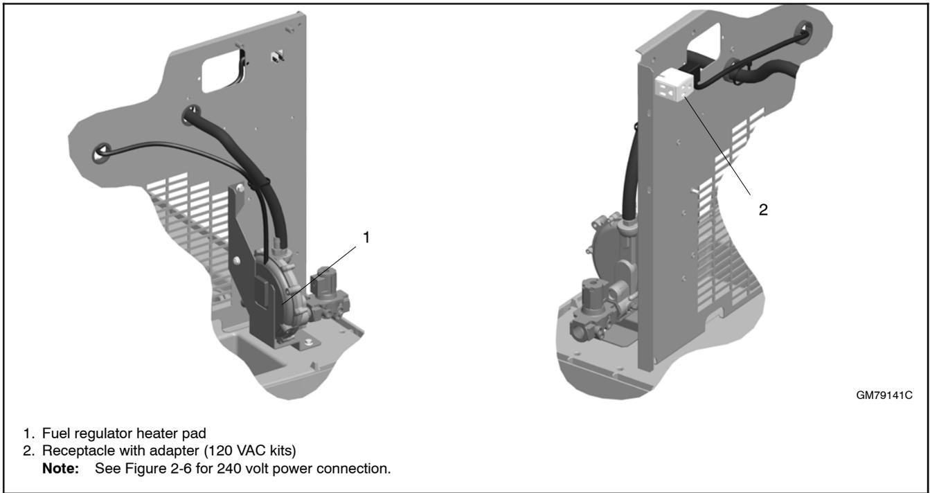
**Figure 2-7** Installed Regulator Heater Kit (for 20RESA/RESAL/RESC/RESCL)
