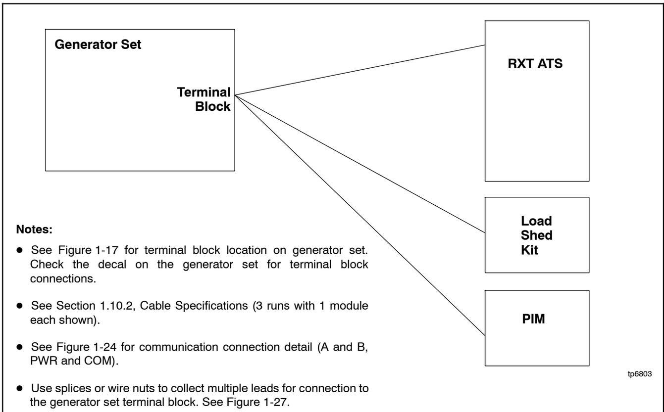
**Figure 1-26** Accessory Module Connections (three cable runs with one module each)
