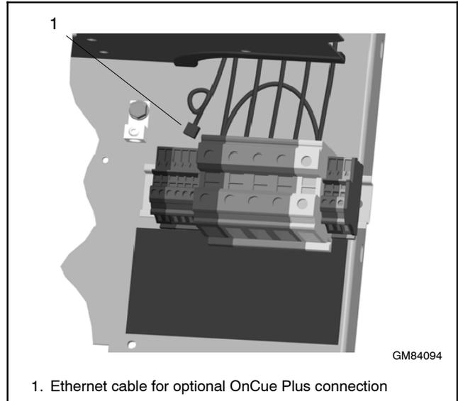
**Figure 2-16** Network Connection for OnCue Plus
