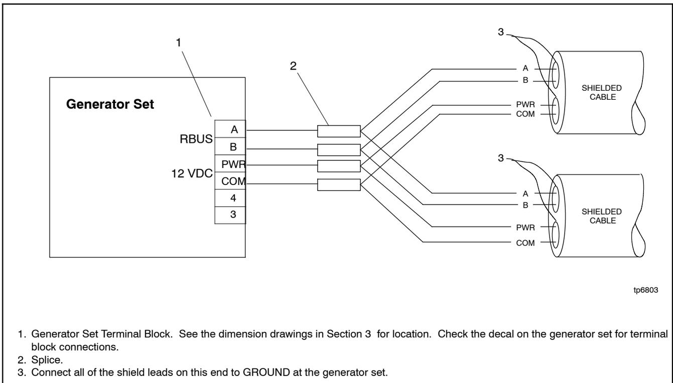
**Figure 1-27** Multiple Connections to the Generator Set
