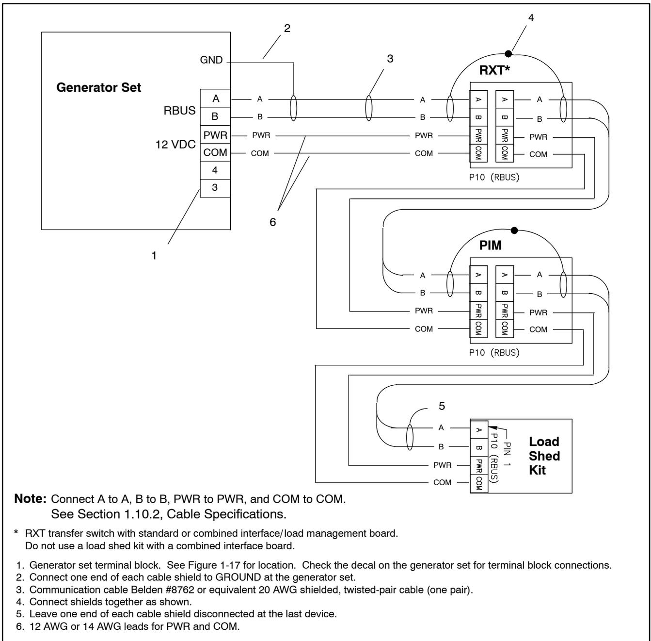
**Figure 1-25** Accessory Module Connections with 12-14 AWG Power Leads
