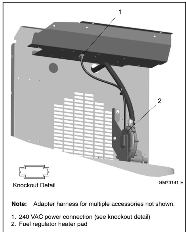
**Figure 2-6** Model 20RESA/RESAL/RESC/RESCL 240 Volt Kit Power Connection
