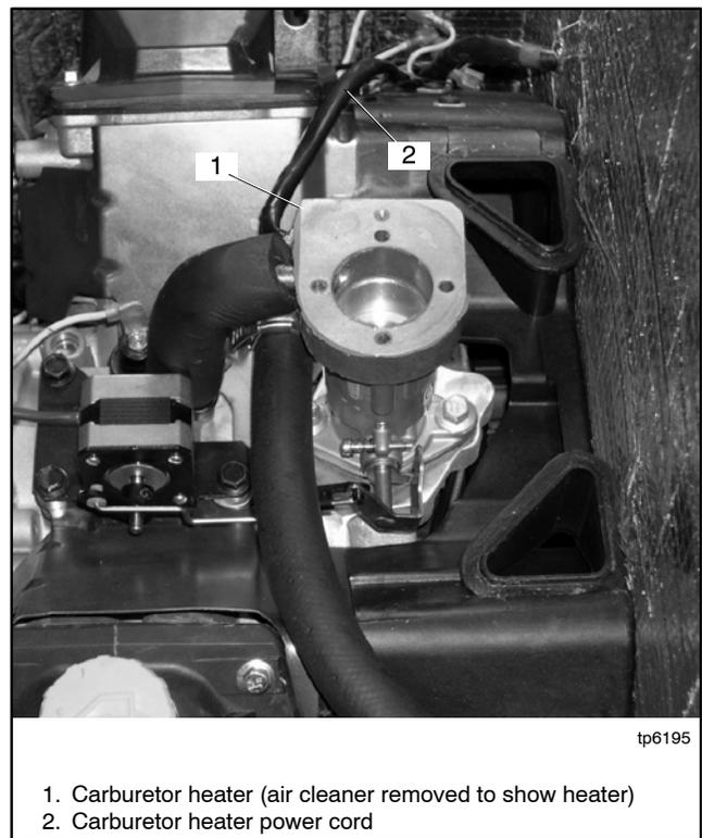
**Figure 2-10** Carburetor Heater for 14 kW Models
