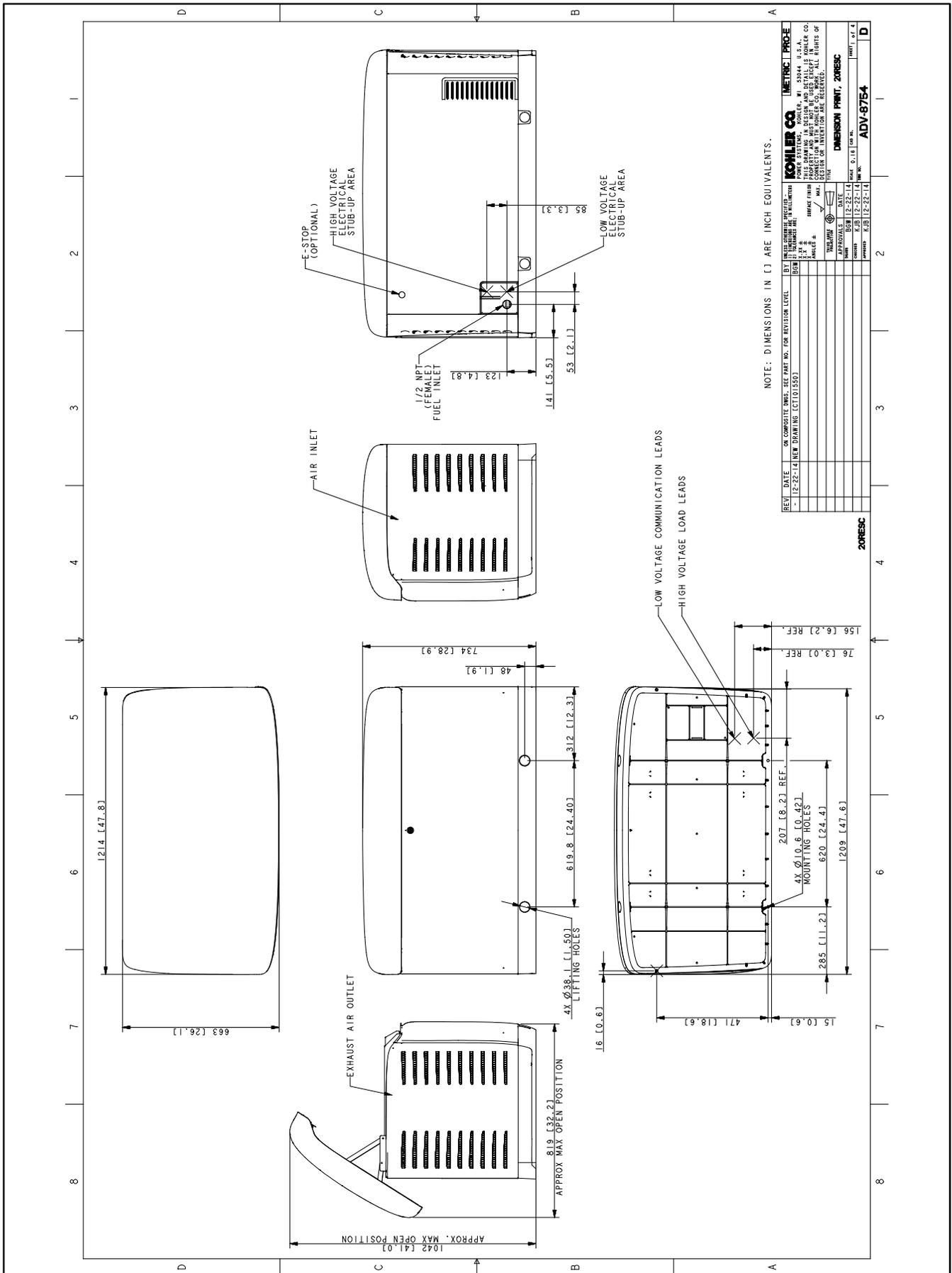
Figure 3-7 Dimension Drawing, Model 20RESC/20RESCL, ADV-8754, Sheet 1 of 4
