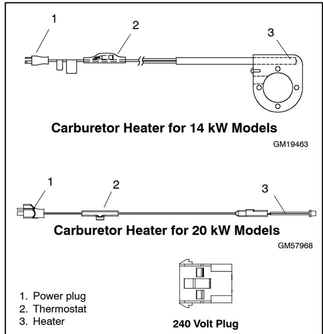
**Figure 2-9** Carburetor Heaters
